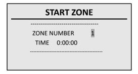
Enter the zone number and the required run time. Press the "OK/Select" key.
