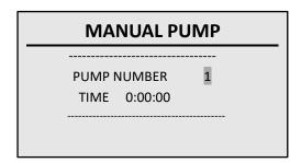
Enter the pump number and the time you want to run the pump for in hours, minutes and seconds. Press the "**OK/Select**" key.
