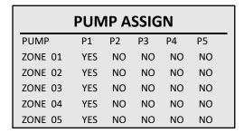
To assign a pump to a particular zone, position the cursor over the relevant field and press the "**OK/Select"** key. "**NO**" will change to "**YES**".
