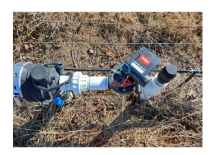
Richard really liked that the Tempus® Ag system could be run via his PC, phone or tablet. The software and app were easy to use and with the in-field battery controllers having an 800m radio radius back to the Wi-Fi Gateway in his office, all his valves were quickly communicating. Michael says'
